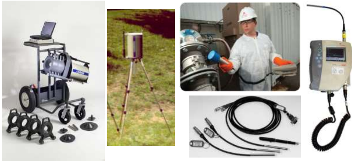
Figure 1 Various In-situ measurement instruments: ISOCS shield set and detector, Ge detector on tripod, scintillation detector with InInspector1000 MCA, collection of small CZT probes, and InInspector1000 with small CZT probe attached.
